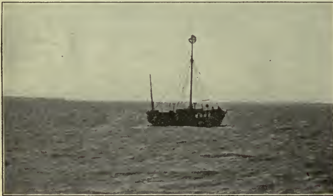
FIG. 69. — A lightship on which men live, keeping the light on the mast burning at night, and the fog whistle blowing in foggy weather.
